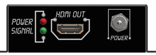
**POWER/SIGNAL LED:** Red light - POWER; Green light - SIGNAL ACTIVE **HDM OUT:** Connects to a HDMI<sup>TM</sup> display with a HDMI<sup>TM</sup> male-male cable here **POWER:** Connects to a 5V DC power supply unit
