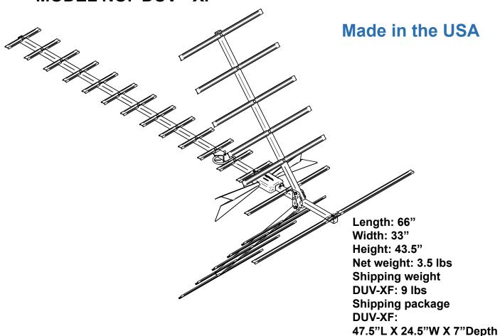
Range: 0 to 80+ miles based on flat open terrain with no obstructions at 30 ft.
